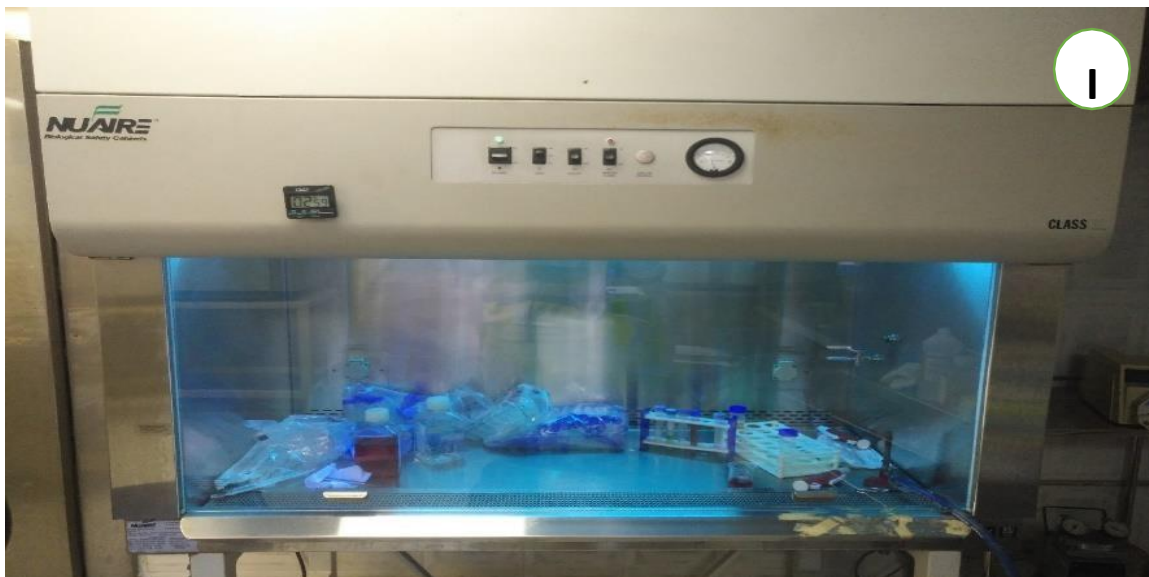
Fig. (15): (A&B) showing components of complete media from left to right; collagenase, Dulbecco's modified Eagle's medium DMEM and phosphate-buffered saline PBS (C&D) harvested tissue in petri dish and Falcon flasks (E&F) examination of stem cells under microscope (G) centrifuge (H) incubation of cells in the incubator (I): air laminar flow safety cabinet
