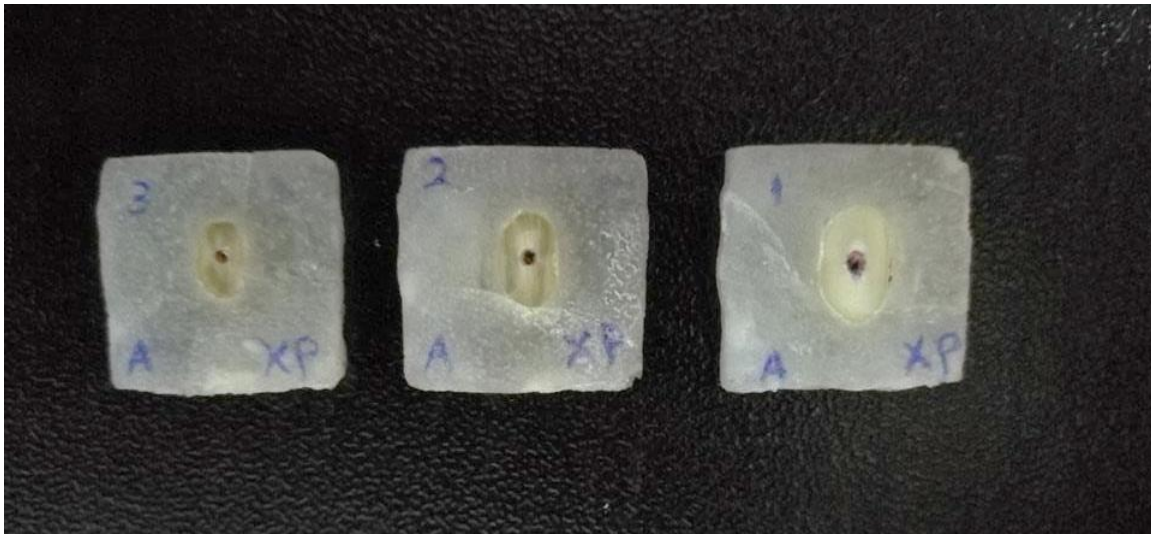
Figure (22): A photograph showing the apical view of the Ad XP-F specimens after pushing of the root canal filling material.
