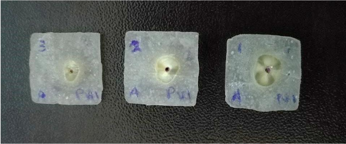
Figure (24): A photograph showing the apical view of the Ad PUI specimens after pushing of the root canal filling material.
