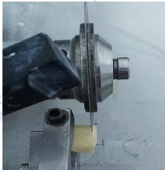
Figure (12): A photograph showing isomet disc during horizontal sectioning of the block.
