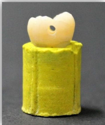
Fig. (16): A photograph showing drilled holes in the both buccal and lingual walls.
