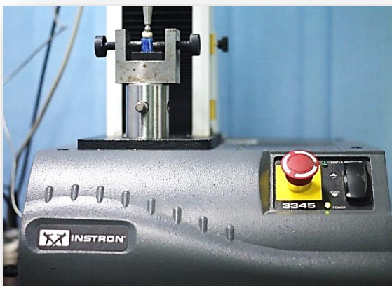
Fig. (24); a photograph showing Instron testing machine.
